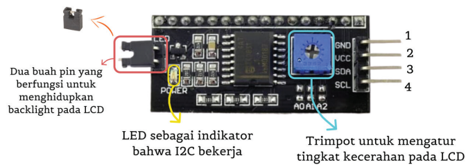
Gambar 9.21 Pin Modul I2C
